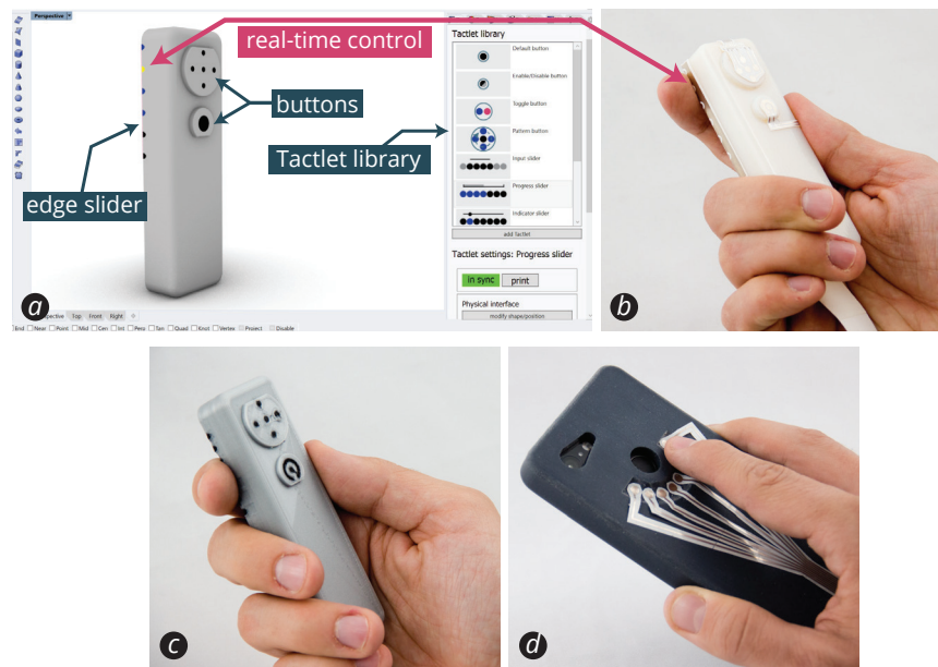
Figure 5.1: Tactlets is a novel approach enabling digital design and rapid printing of custom, high-resolution controls for tactile output with integrated touch sensing on interactive objects. (a) A design tool allows a designer to add Tactlet controls from a library and customize them for 3D object geometries. The designer can then fabricate a functional prototype using conductive inkjet printing (b) or 3D printing (c), and explore the interactive behavior of the Tactlet control. (d) This approach allows for rapid design iterations to prototype tactile input and output on a variety of objects.
