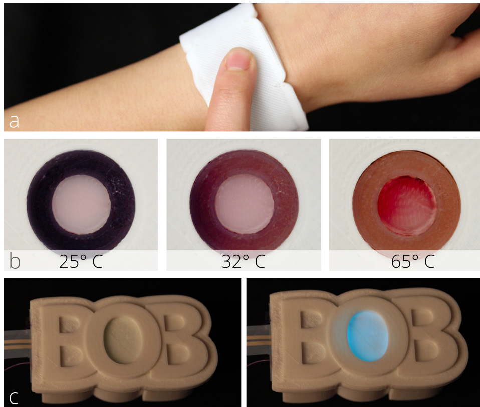
Figure 6.3: Embedded input and output modalities: a) capacitive touch sensing, b) thermochromic display, and c) thin-film display.
