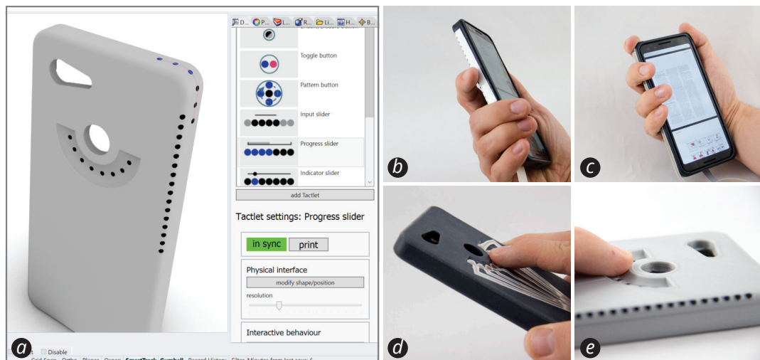
Figure 5.13: Application case 1: Through several iterations different slider Tactlets are quickly prototyped on a smart phone case. (a) Three tactlets are digitally designed in the design tool. (b) A long slider on a curved edge on the back of the case, (c) a short slider wrapped around the top left curvature, and (d & e) a curved concave slider on the back of smart phone case as (d) inkjet-printed and (e) 3D-printed prototype.
