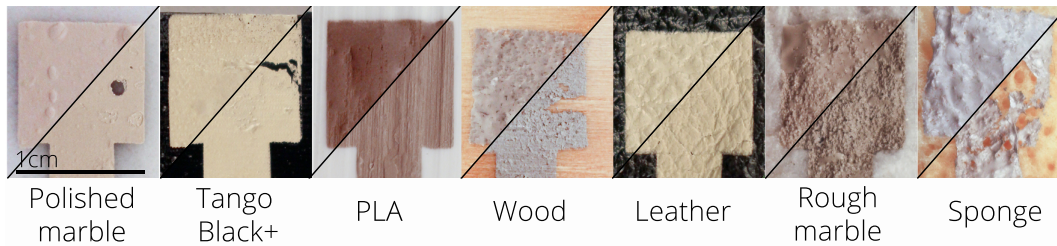
Figure 4.3: Materials. Top left: sample covered with transparent PVA transfer film, bottom right: after washing the PVA transfer film off.
