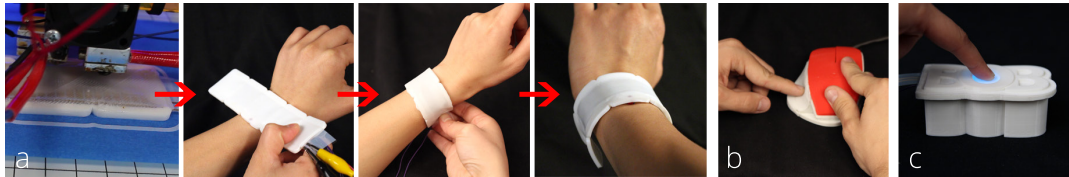
Figure 6.1: a) 3D-printed object with embedded state-changing elements. The end-user can physically customize the object on-demand after it is fabricated. This enables user-tailored wearables, b) ergonomically personalized devices, and c) new kinds of interactive objects.
