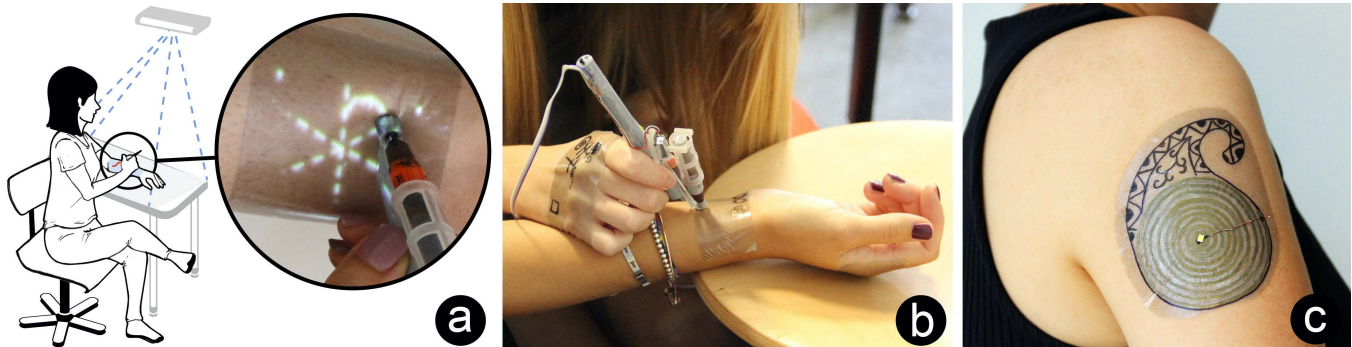
Figure 1: BodyStylus combines design and fabrication of functional on-body interfaces into one integrated activity performed directly on the body. A handheld device combines the ease and directness of free-form drawing with digital assistance; visual cues provide guidance while constraints dynamically restrict inking to prevent errors. BodyStylus enables drawing on one's own body (a), as well as collaborative design (b), to realize functional epidermal interfaces (c).
