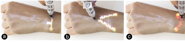
Figure 10: Parametric components. The user places a bend sensor design on the wrist (a) and enhances its visual aesthetic with a curlicue pattern. She drags the center, which modifies the pattern on-the-fly (b). When moving the sensor to a body location the user cannot bend, the body constraint is highlighted in red (c).
