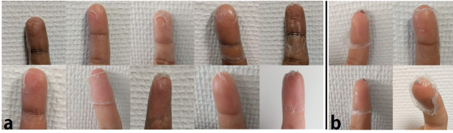
Figure 10: (a) Patches of the Low RIGIDITY condition were damaged during the surface discrimination task for 10 participants. (b) 4 patches of the Medium Rigidity condition were damaged.
