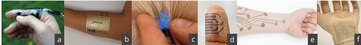
Fig. 1. Examples of Epidermal Computing Devices for a) eyes-free touch input [230], b) wireless communication through aesthetic on-skin tattoos [97], c) displaying notifications through ultra-thin displays [232], d) feel-through haptics [234], e) sensing physiological signals [155] and f) skin stretchable large scale transistor array for on-skin computing [225]
