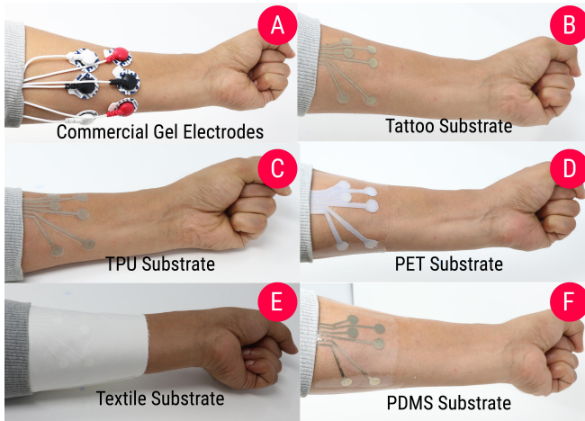
Figure 3. Conformal skin contact made by the electrodes fabricated on all the substrates.
