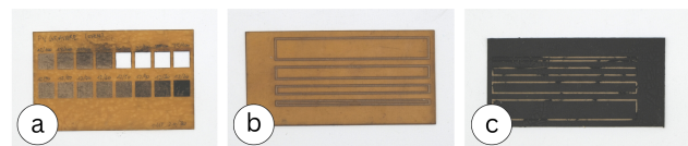
Figure 11: Carbonization tests: a) master sample with power/speed ratios, b) 12W 10mm/s ablation on simple BC sample and c) 12W 10mm/s ablation on the graphite-imbued sample.
