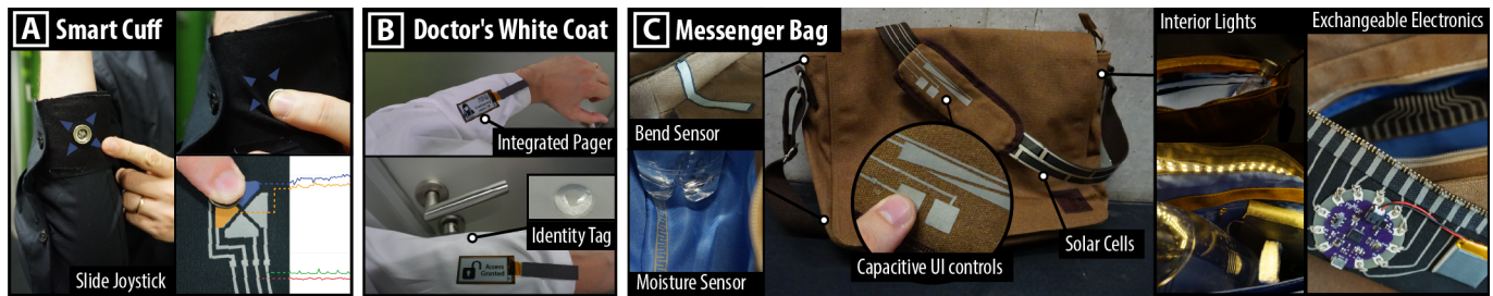
Figure 11. We present the three application examples of a Smart Cuff for Business Presentations (A), a Doctor's White Coat (B) and a Messenger Bag (C).
