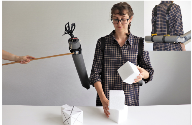
Figure 2: Study setup with the WRA form factor prototype. The backpack-worn arm is made of foam tubes, a basic gripper, and one articulated joint. The experimenter uses a stick to control it.
