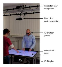
Figure 2. Prototypical implementation of Permulin
