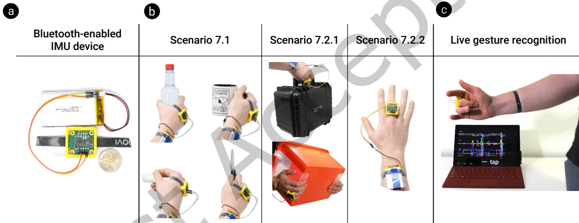
Fig. 22. Minimal wireless hardware with battery a); scenarios involving multiple objects and freehand b); live classification of gestures c).
