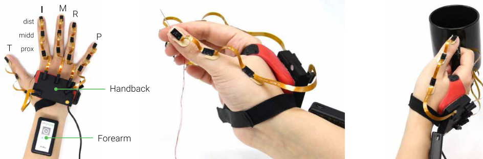
Fig. 2. Hardware setup with 17 synchronized IMUs placed all over the dominant hand. It preserves cutaneous properties and allows unobtrusive interaction with complex object geometries. The left image labels describe the spatial notation of each IMU used in our analysis.
