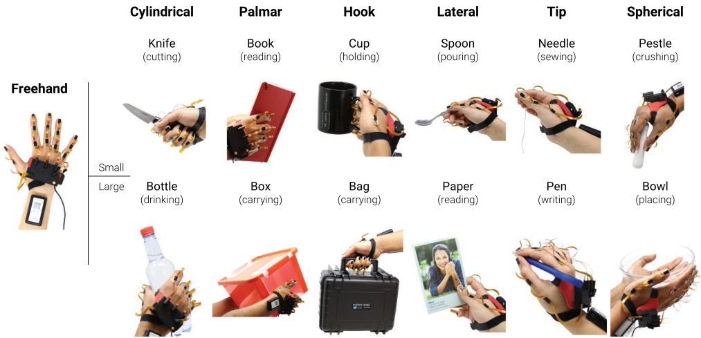
Fig. 3. Using a dense network of 17 IMUs placed on the hand, the microgestures dataset was collected for Freehand and while Grasping 12 objects covering each of the six grasp types with two variations.
