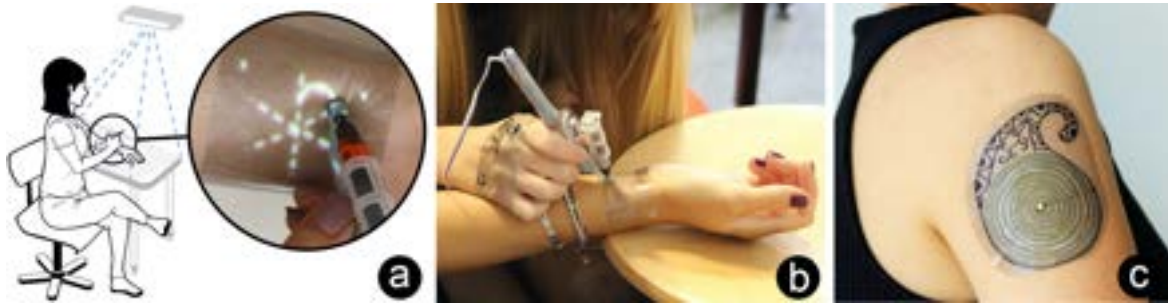
Figure 3.1 BodyStylus combines the design and fabrication of functional on-body interfaces into one integrated activity performed directly on the body. A handheld device combines the ease and directness of free-form drawing with digital assistance; visual cues provide guidance while constraints dynamically restrict inking to prevent errors. BodyStylus enables drawing on one’s own body (a), as well as collaborative design (b), to realize functional epidermal interfaces (c).
