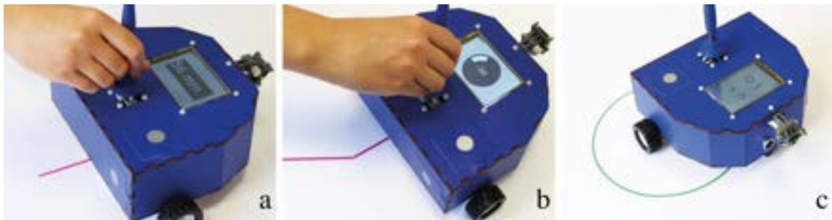
Figure 5.10 RoboSketch as a tool for a) linear measurement, b) angular measurement, c) and drawing guidelines.
