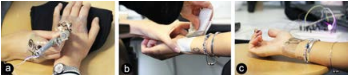
Figure 3.15 Artists during focus group exploration. Inking on each other (a), applying substrate for functional prototype interface (b), completed epidermal interface controlling an RGB LED (c).
