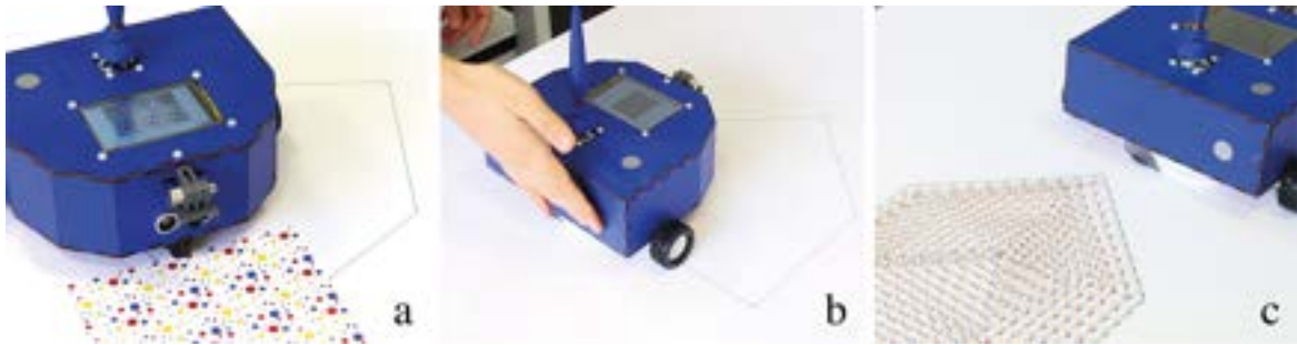
Figure 5.8 Coloring a shape: a) scanning the desired color/pattern, b) placing the robot on the shape's contour, c) robot fills the shape with the color/pattern.
