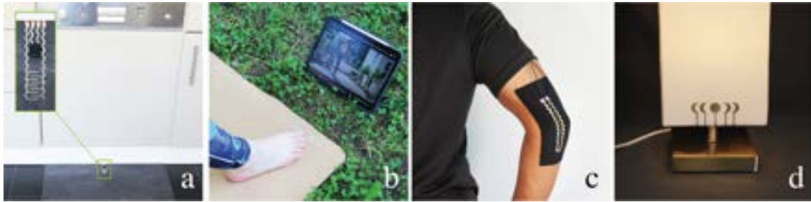
Figure 4.20 Application examples demonstrate the practical feasibility and applicability of our technique on everyday surfaces: a) moisture sensor on a floor tile, b) interactive yoga mat, c) wearable stretch sensor on kinesiology tape, and c) capacitive slider on a table lamp.
