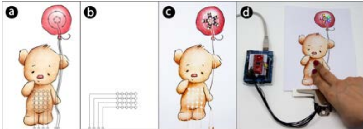
Figure 6.14 Interactive greeting card: (a) Front side of the greeting card with dot patterns highlighting the sensor area, (b) backside of the card, (c) fabricated card contains hand-drawn multi-touch sensor and LEDs, (d) the sensor is connected to an Arduino Uno with a clip.
