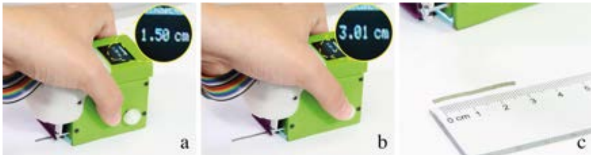
Figure 4.15 Print-A-Sketch as measurement tool: a-b) the display visualizes the length of the printed trace, c) shows the accuracy of the printed trace.
