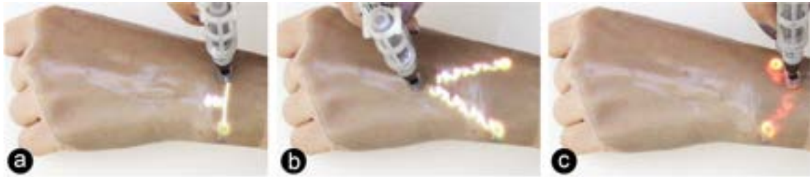
Figure 3.10 Parametric components. The user places a bend sensor design on the wrist (a) and enhances its visual aesthetic with a curlicue pattern. She drags the center, which modifies the pattern on-the-fly (b). When moving the sensor to a body location the user cannot bend, the body constraint is highlighted in red (c).
