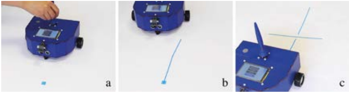
Figure 5.5 Routing toward existing mark: a) guiding the robot toward the desired direction, b) the robot detects the mark and connects the trace, c) the robot stops printing before reaching a trace and continues afterward, or can autonomously route around small visual elements.
