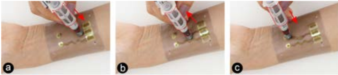
Figure 3.7 Constraints prevent invalid connections of conductive traces. The user draws a conductive trace to connect two terminals (a). As she is about to connect to another conductive trace and create a short circuit, the pen retracts to non-inking mode (b). Moving the pen away from the original trace switches the pen back to inking mode (c).
