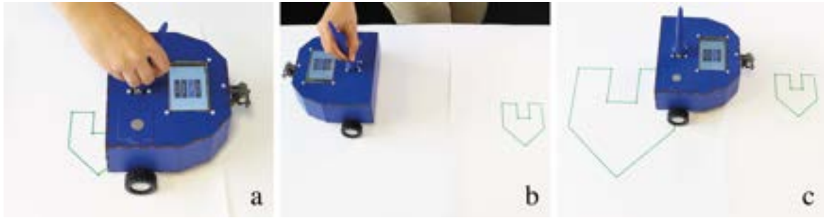
Figure 5.6 Scaling a design: a) sketching a small scale design in manual mode, b) defining the desired scale in assisted mode, c) robot sketches the scaled-up design in autonomous mode.
