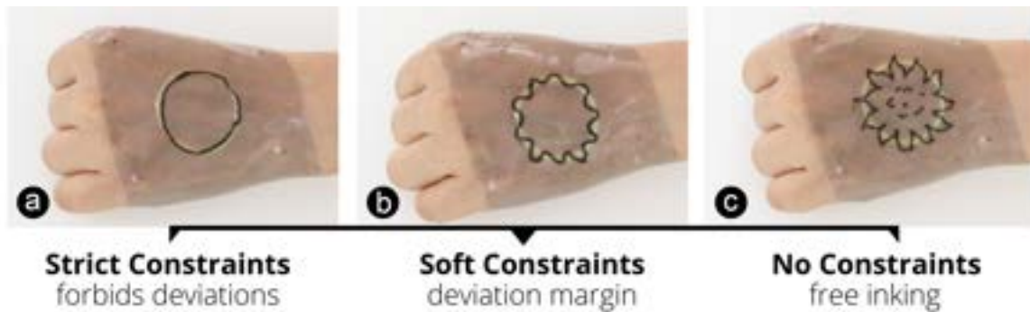
Figure 3.4 Constraints can be imposed at different levels. In this example, a strict constraint forces the user to closely follow the projected shape primitive (yellow circle, a). A soft constraint allows the user to deviate within a certain margin, for creative adjustments (b). Without constraints imposed, the user can draw freely, while still benefiting from high-level visual guidance (c).
