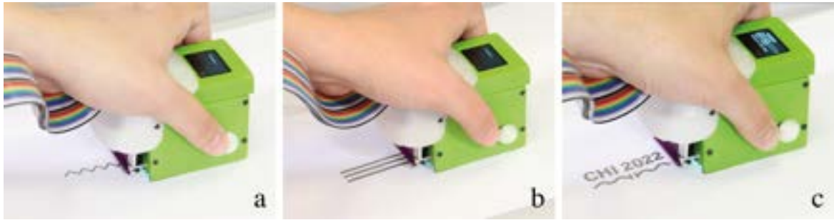
Figure 4.9 Custom Brushes: a) Printing traces with custom pattern and width, b) printing multiple lines, c) stamping an uploaded image.
