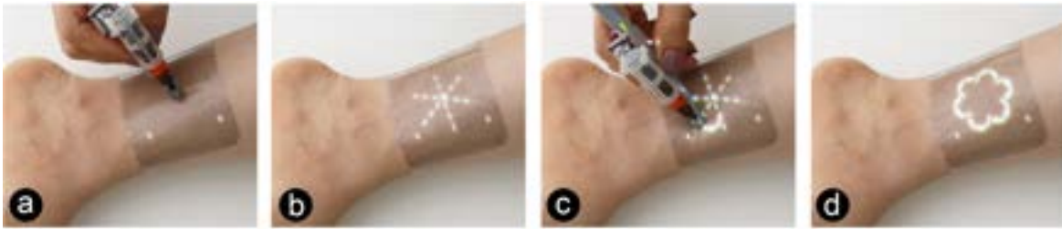
Figure 3.6 Radial symmetry tool enabling rapid designs of repeating patterns, building on practices from henna art. The user positions the center of the symmetry axes (a), and these axes appear as guides (b), the user draws the geometrical pattern in one sector (c), and the pattern is replicated in the other sectors (d).
