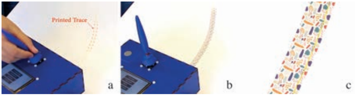
Figure 5.7 Refining: a) sketching a trace in light color, b) robot revisits and refines the trace with the desired pattern, c) close-up view of the pattern.
