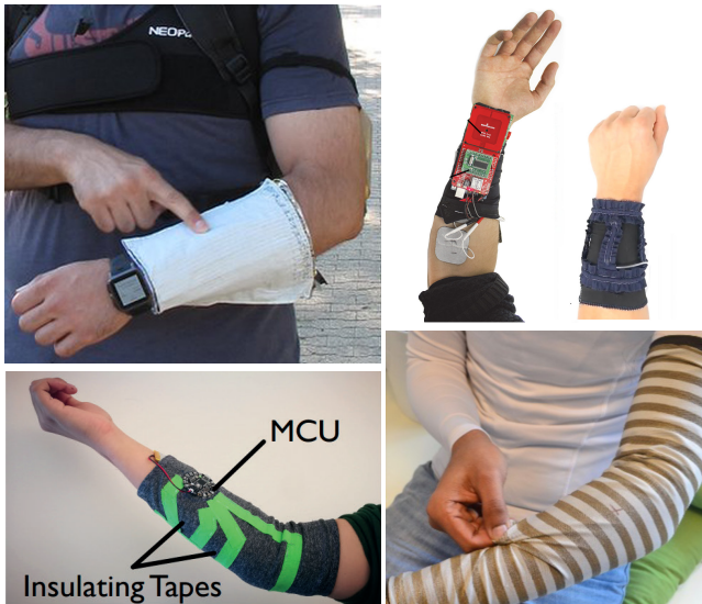
Figure 3: Examples of existing wearable sleeves. Top: GestureSleeve [68], Affordances++ [37] and PneuSleeve [81]. Bottom: Textile for reconstructing joint angles [34] and SmartSleeve [49]
