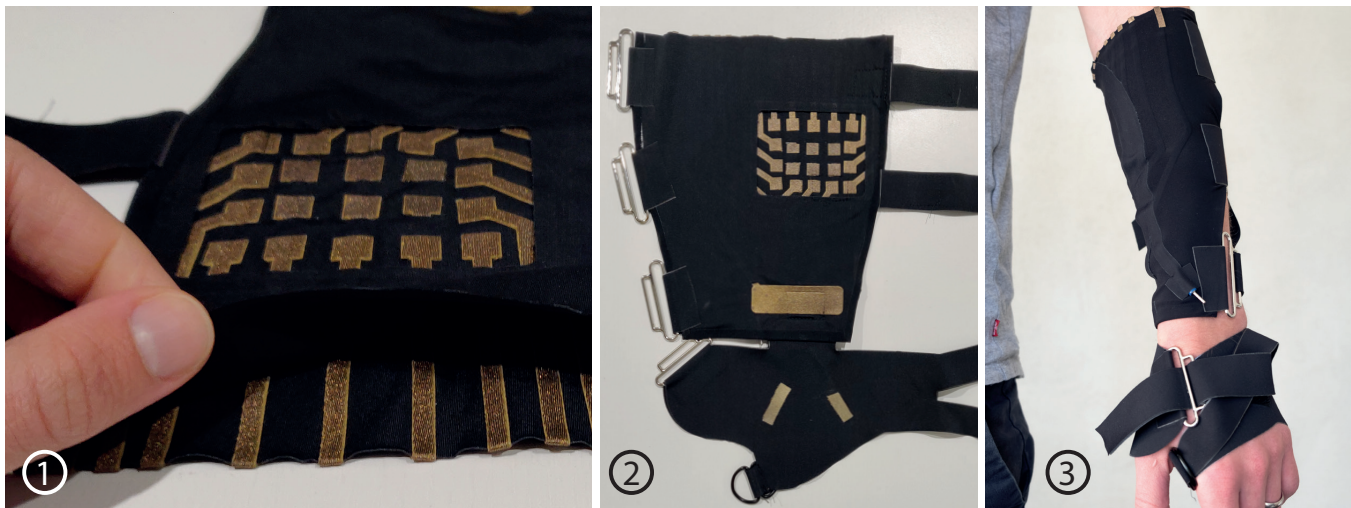
Figure 8: The Typing Sleeve. (1) This sleeve features an array of 20 small electrodes in a grid-like pattern, with fabric traces routing primarily between layers of base fabric. (2) The sleeve also features a large wrist ground electrode, and two palm electrodes on a half glove. (3) Cummerbund and d-ring fasteners are used to fasten the sleeve to the arm.
