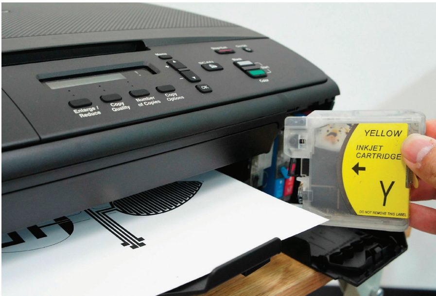
Figure 1. Using a consumer-grade inkjet printer to print a conductive circuit on photo paper [1]. (Courtesy of Yoshihiro Kawahara)
