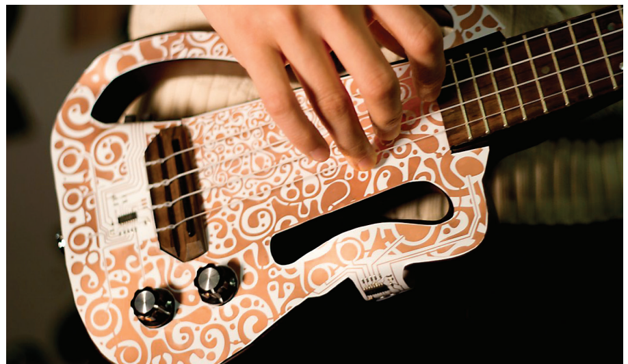
Figure 2. Printed circuits can be both functional and aesthetic. This is a capacitive sensor for music control on an electric ukulele, adapted from an artwork by Evgeny Kiselev. (Courtesy of Nan-Wei Gong)
