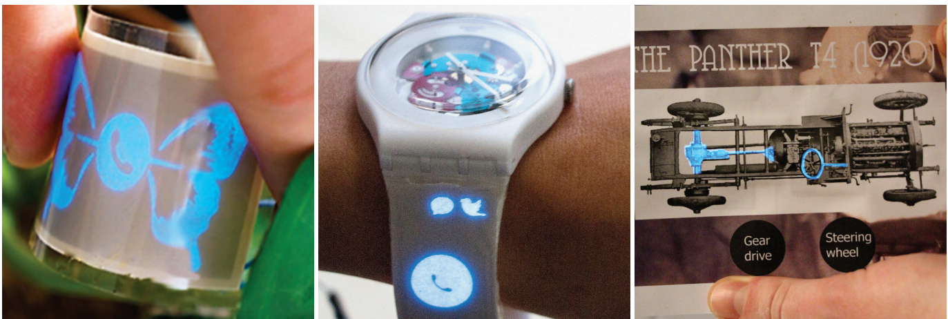
Figure 4. Some examples of deformable touch-sensitive displays fabricated with PrintScreen [6].
