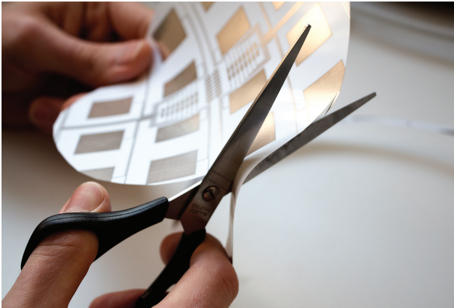
Figure 3. This multi-touch sensor sheet is cuttable into various shapes and remains functional. This enables physical prototyping of electronic components [4].
