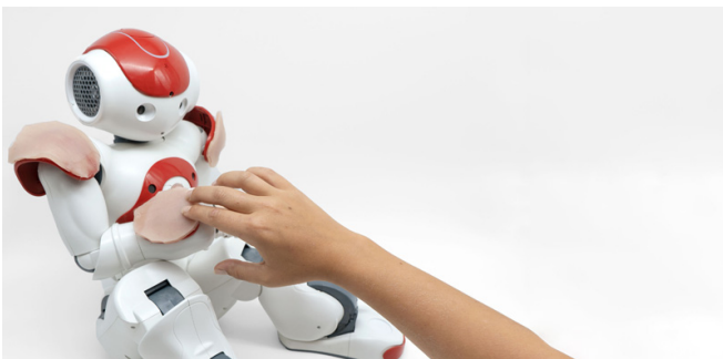
Fig. 11: The sensor can be shaped to conform to any robot. Here, a skin sensor is attached to a Nao social robot.
